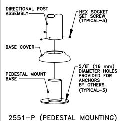
**REMOVABLE** DIRECTIONAL POST **BOLLARD ASSEMBLY** HOLE COVER AVAILABLE ON REQUEST 0'-0" FINISHED GRADE NOTE: CONCRETE FOOTING AND NO. 4 REBAR (BY OTHERS) PER LOCAL SOIL Δ REMOVABLE BOLLARD INSERT CONDITIONS.
